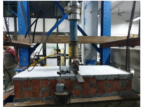
Figure 4: Test setup of the flexural test for all specimens.
