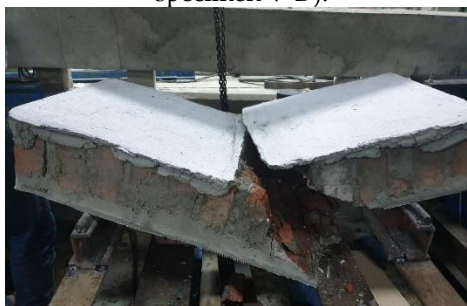
c- Third failure mode (shear failure for specimen H-D).
