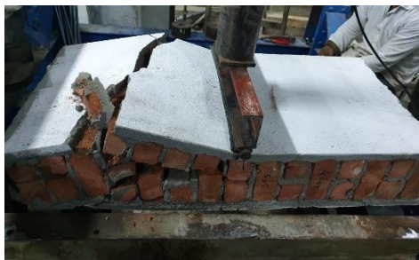
b- Second failure mode (compression failure for specimen V-D).
