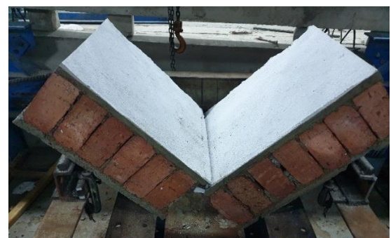
a-First failure mode (tension failure).
